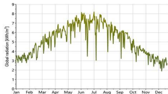
Fig. 3. The solar radiation profile for one year.
